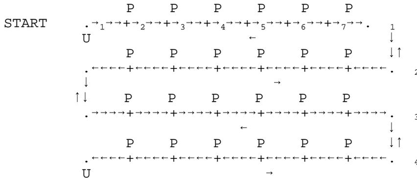
**EXAMPLE #7,** One axis, 20 bytes RAM: Homing and looping using loop-marker
