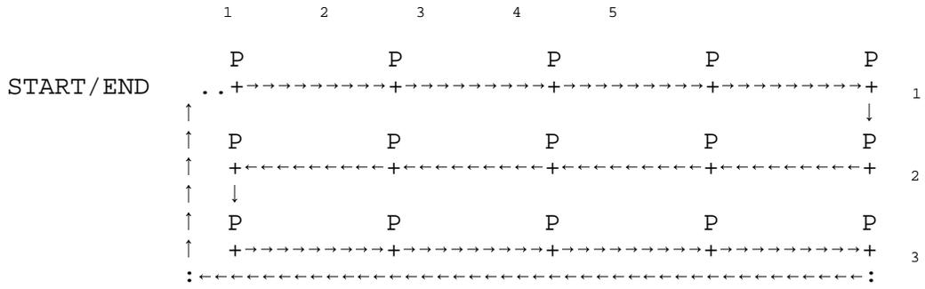
**EXAMPLE #5,** Two Axis, 17 bytes RAM: Mirror-image X,Y Matrix
