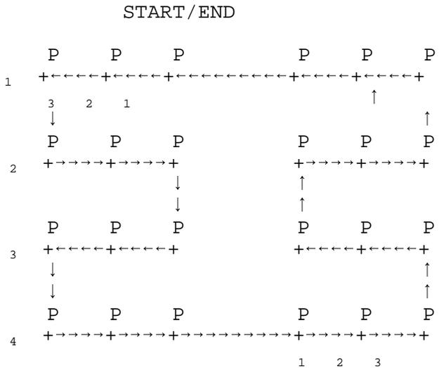
**EXAMPLE #6,** Two Axis, 17 bytes RAM: Raster Scan with 20 usec output pulses
