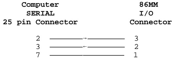
If a shielded cable is used, connect the shield to connection 12 on the 86MM I/O.
