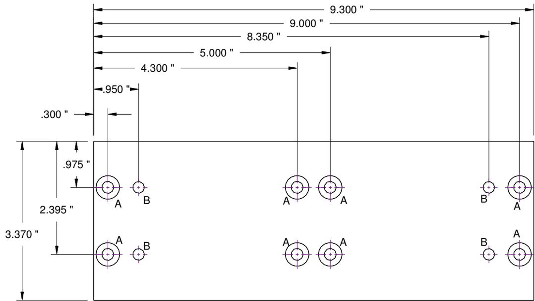
A Counter bore for 1/4-20 Button Head .257 " thru
