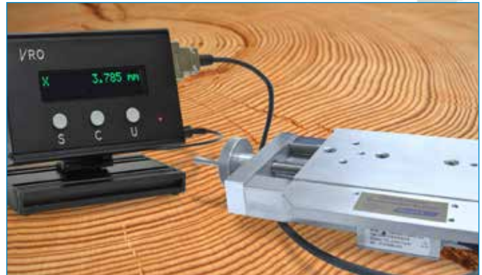
Velmex’s TA System has been recognized by North America’s Dendrological Research Community. It includes the proven UniSlide Assembly to maneuver the cookie or core under the microscope.
