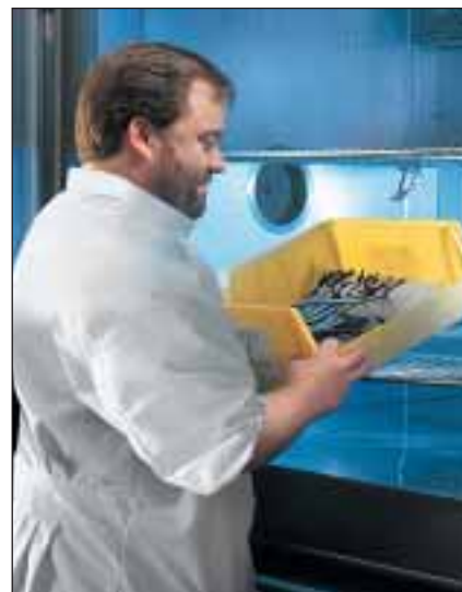
Environmental test chamber ensures that all reading heads can withstand extremes in temperature and humidity.
