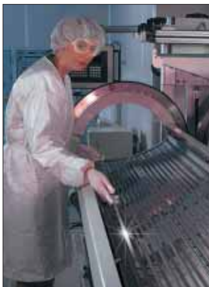
Vacuum coating equipment ensures consistent chromium deposition.
