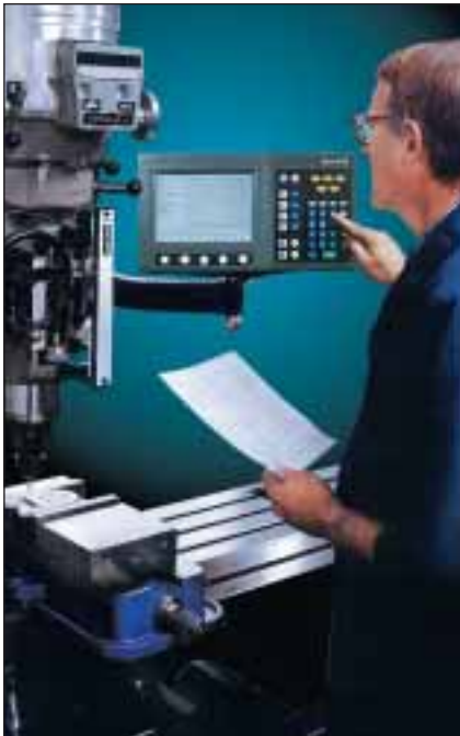
ACU-RITE Readout Systems accurately measure machine movements and communicate this information to the operator in a clear, concise manner.
