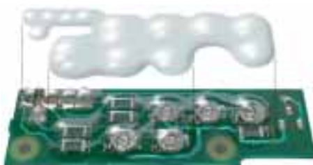
Conformal coating is applied for extra protection.
