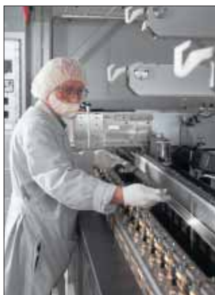
Scale-replicating equipment in a Class 100 clean room environment.
