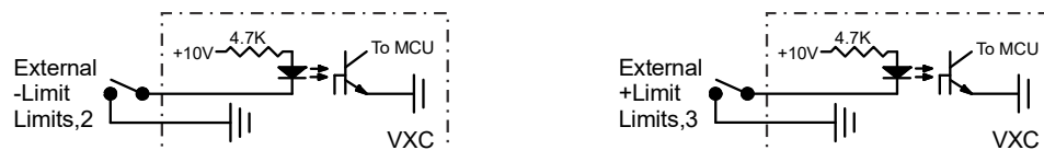
Figure 4 Limit Switch Input Hardware
